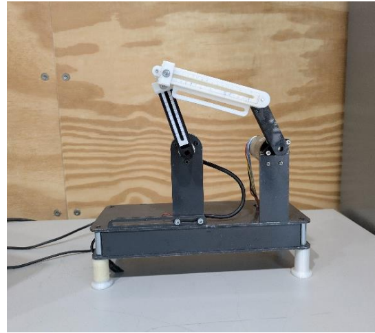
Figure 11. Experimental platform overview with different links lengths and configurations
